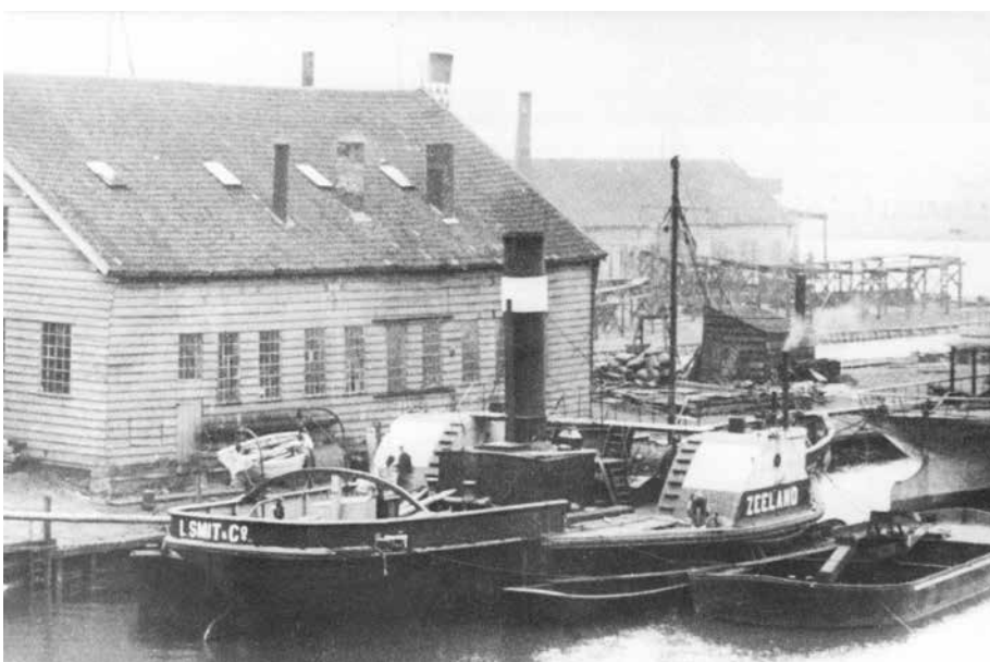
The paddle tug ZEELAND - the second of that name - was built in 1868 by L. Smit & Zn, Kinderdijk, for account of Stoomsleepdienst L. Smit & Co., Alblasserdam, later Rotterdam. 33,53 x 12,08 (oa) / 6,65 (hull) x 3,05 m. Draft 2,00 m. Iron hull. 1874 re-engined, 260 ihp. 1908 converted to non-propelled salvage vessel. 1917 sold for scrap photo: coll. Job van Eijk
