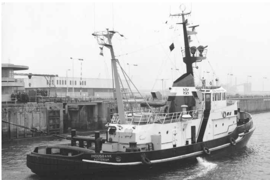
The Voith Tractor INDUSBANK was fully fitted for salvage and rescue operations in the North Sea
