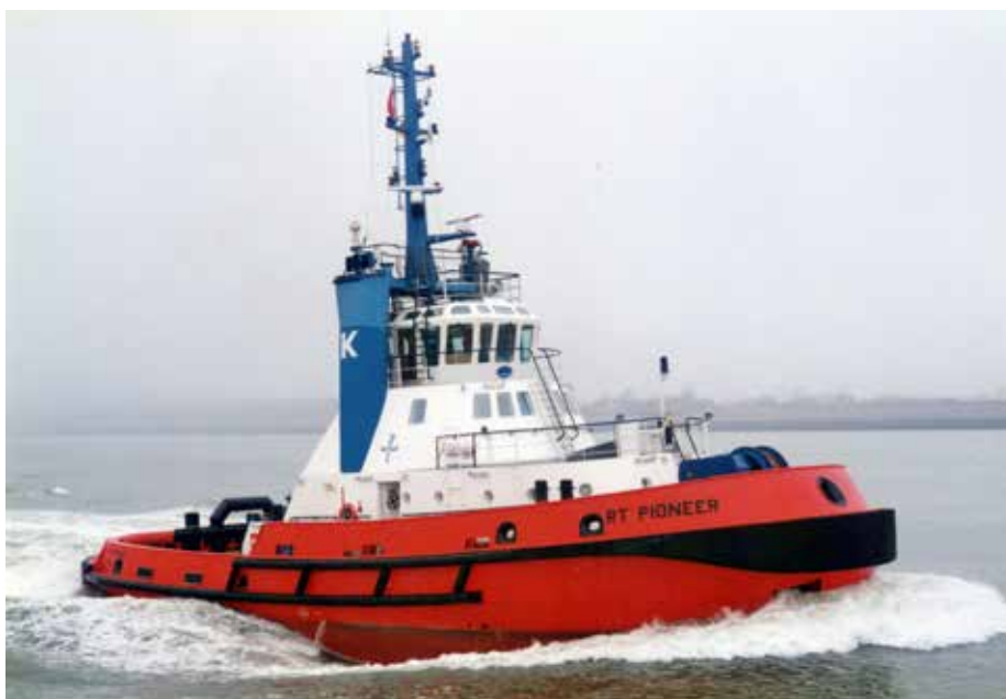
RT PIONEER was the first of four 'Rotor Tugs' developed by Kooren
