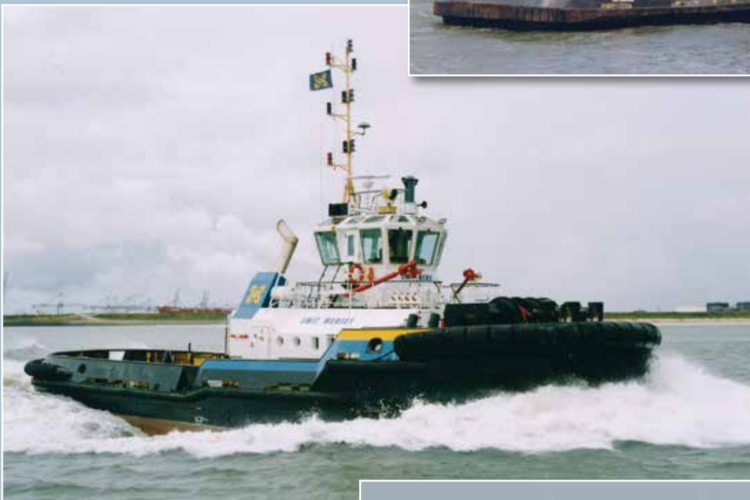
Third generation Rotterdam shiphandling tug: reverse tractor tug designed by Damen Shipyards: SMIT MERSEY built 1999. 4.908 bhp - 61,3 ttp. 2009 renamed SMIT NIDA operating in Lithuania. 2013 to Smit Lamnalco as SL NIDA. 2019 sold to Canada as DALTON WARRIOR. Delivery trip was under the name of IDA 1
