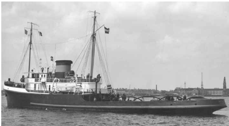
ZWARTE ZEE was built for L. Smit in 1933. The first motor tug in the fleet and at the time the most powerful in the world (3.200 bhp / 4.000 hp - speed 17 knots). The main engines were Werkspoor from a new untested model designed by ir Lugt. 10 May 1940 escaped to England towing the half-finished destroyer ISAAC SWEERS. 20-8-1940 bombed at Falmouth and partially sunk. Repaired and in service as Rescue Tug W 163. 1951 damaged in collision. 1961 renamed ZWARTE ZEE III . 1962 RENAMED IERSE ZEE . 1966 sold to Frank Rijdsdijk for scrap
